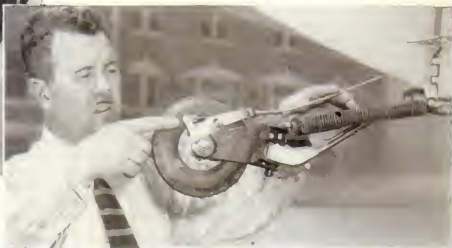
A two-finger lever control in the plane's cockpit sets the tail-wheel brake seen at right, for a quick stop
